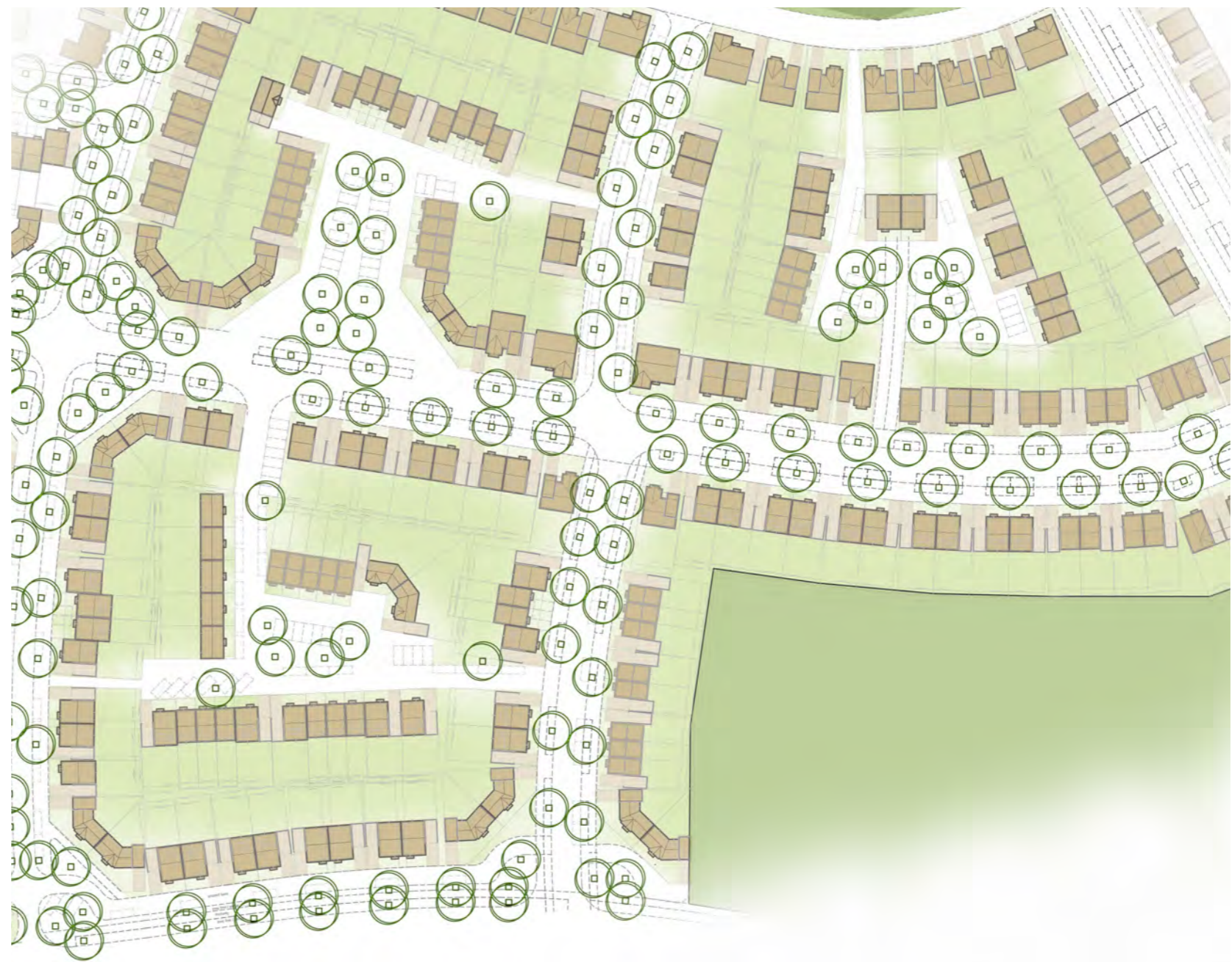
Figure 13.8 Illustrative capacity testing layout for a medium density area at c.34 dph
