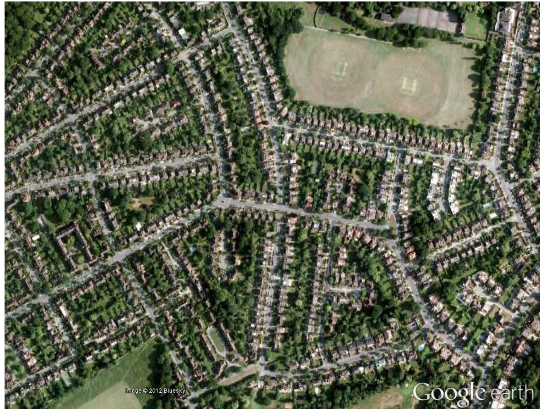
Hampstead Garden suburb aerial view showing a perimeter block structure with enclosed gardens and cul-de-sacs within some of the larger development blocks
