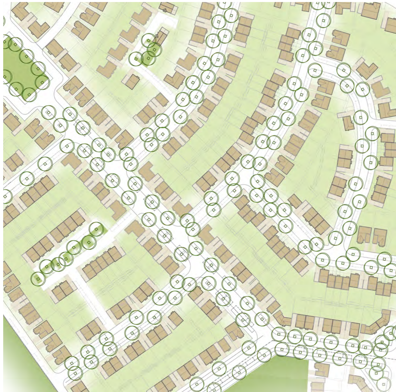
Figure 13.9 Illustrative capacity testing layout for a lower density area at c.27 dph
