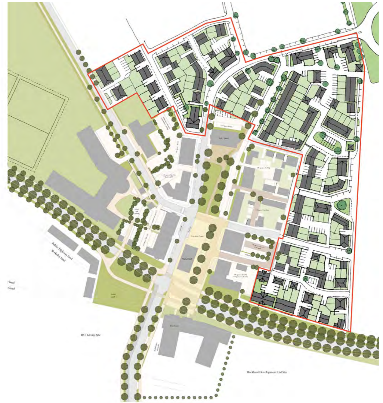
Figure 13.10 Illustrative capacity testing layout for a higher density area at c.42 dph
